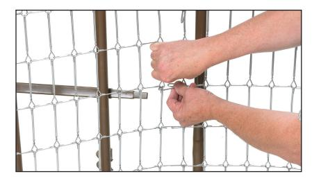
4. Connect head section and foot section by squeezing together and attaching with spring links. Pull up the head section and foot section to release tension between the springs.
