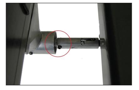
Make sure the slot on the spring loaded shaft engages the roll pin on the gear box.
