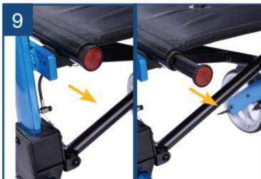
To attach storage bag, pull out the red reflectors located on the front of the seat frame.
