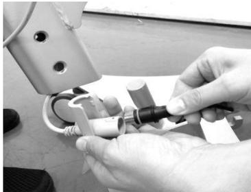
3. Fit the mast into the base socket.
