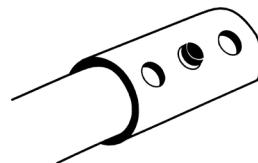
1. Before use, adjust height of each leg to your specific needs, making sure all legs are at the same height. When desired height is reached, lock legs into place by aligning buttons into proper holes, per illustration above.
